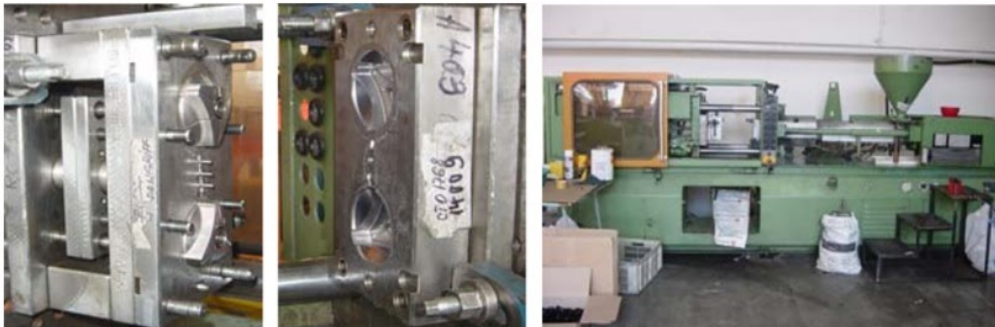
Injection molding machine and punch made at TUCN at work
